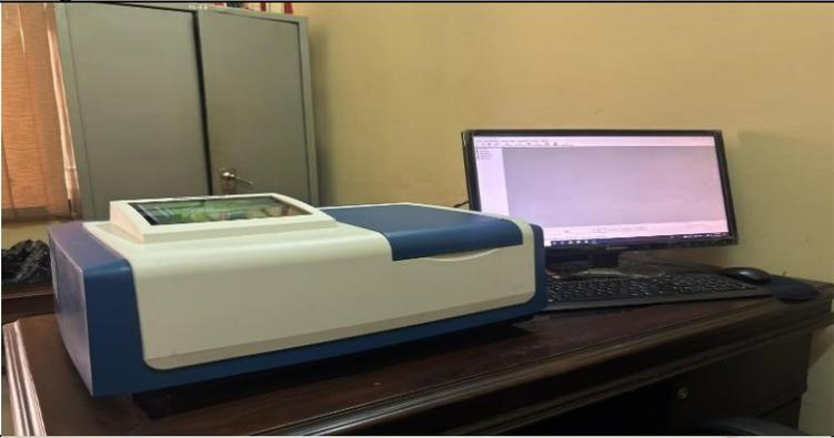
A double beam UV-VIS spectrophotometer, primarily white with blue accents, is positioned on a dark wooden desk. To its right, a computer monitor displays a software interface, with a keyboard and mouse also visible on the desk.                                                                                         |
