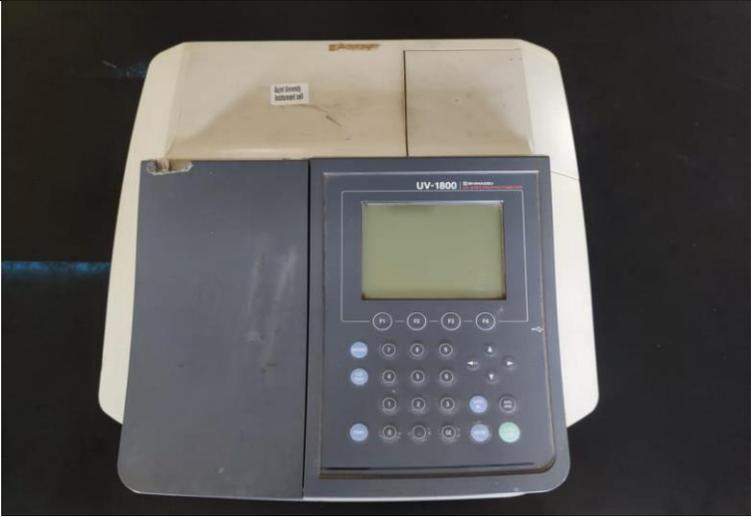
A UV-Vis spectrophotometer, model UV-1800, is shown from a front-facing perspective. It has a white top and a grey control panel with a small LCD screen and a numeric keypad. The brand name 'SHIMADZU' is visible at the top of the instrument.                                                                        |
